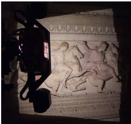
Figure 3: The ATOS III while projecting fringe patterns onto the object
